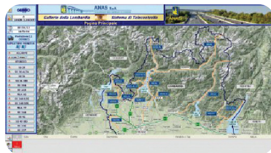
Fig.2 - The supervision and telecontrol system, designed and implemented by Gemmo S.p.A. and based on PcVue SCADA
